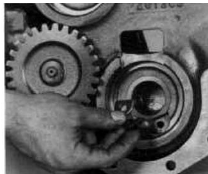
Figure 214 Remove screw and sleeve lock.
