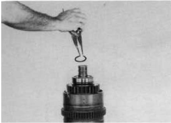
Figure 104 Remove front bearing retainer ring.
