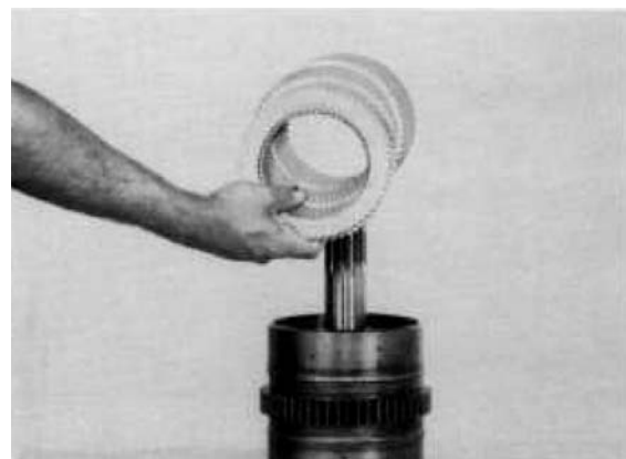
Figure 127 Remove inner and outer clutch discs.
