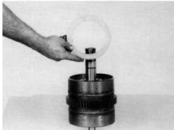
Figure 173 Remove end plate.
