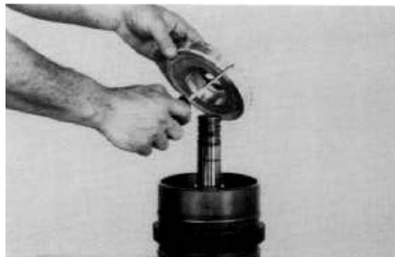
Figure 145 Install clutch piston inner and outer oil seal rings. Install clutch piston in clutch drum, use caution as not to damage seal rings.
