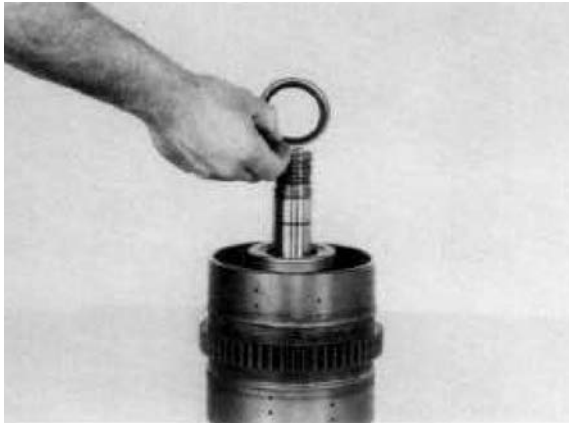
Figure 176 Remove retainer ring retaining ring.
