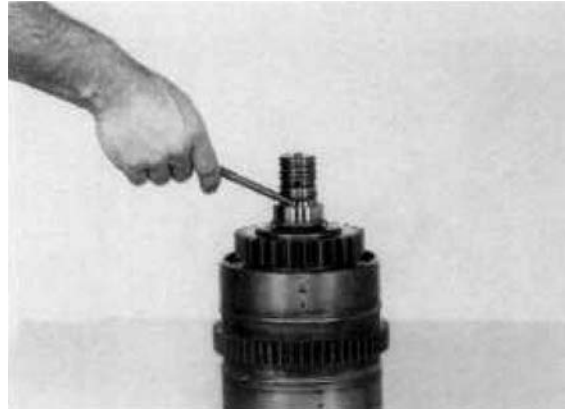
Figure 167 Remove bearing end plate lock ball.
