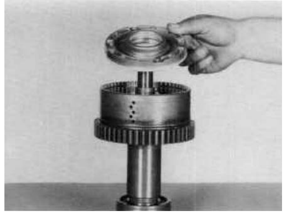
Figure 15 Install new clutch piston inner and outer sealing rings. Insert clutch piston in clutch drum. Use caution as not to damage sealing rings.
