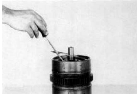
Figure 179 Remove clutch disc end plate retainer ring.
