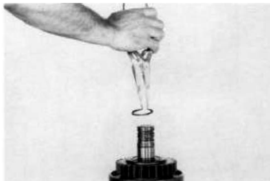
Figure 205 Install bearing retainer ring.
