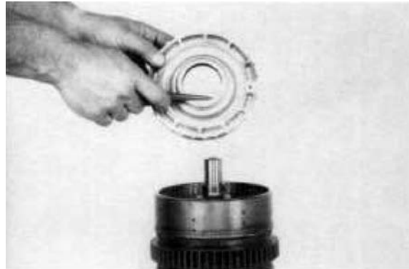
Figure 185 Remove clutch piston.
