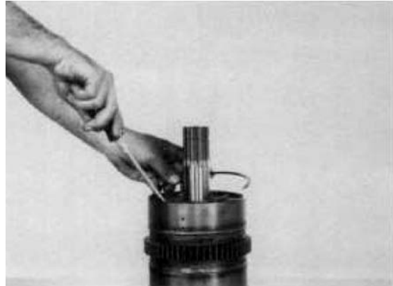
Figure 125 Remove clutch disc end plate retainer ring.
