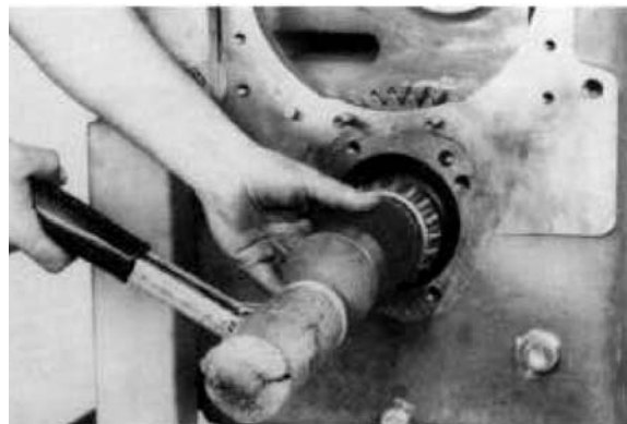
Figure 222 Position output gear in transmission case with protruding hub toward front of case. See Figure 221. Insert output shaft, gear spacer and taper bearing from front of case and through output gear. Install front taper bearing cup. Block output shaft and install rear taper bearing with large diameter in.
