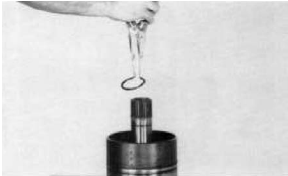
Figure 82 Remove return disc spring retainer ring.
