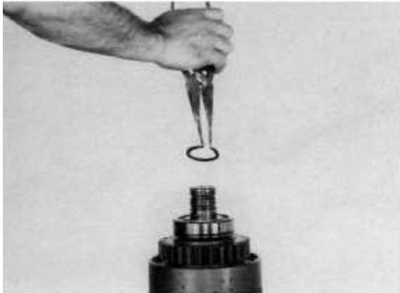
Figure 164 Remove front bearing end plate retainer ring.
