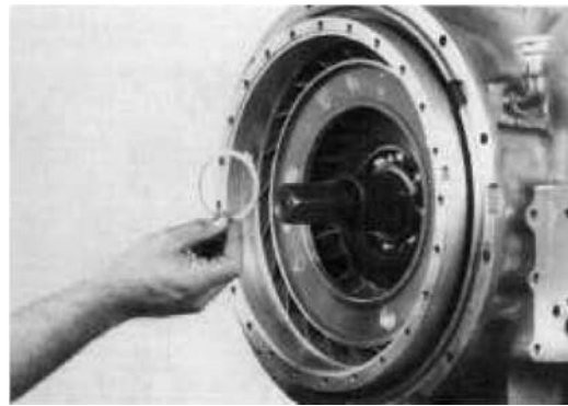
Figure 15 Remove reaction member spacer.
