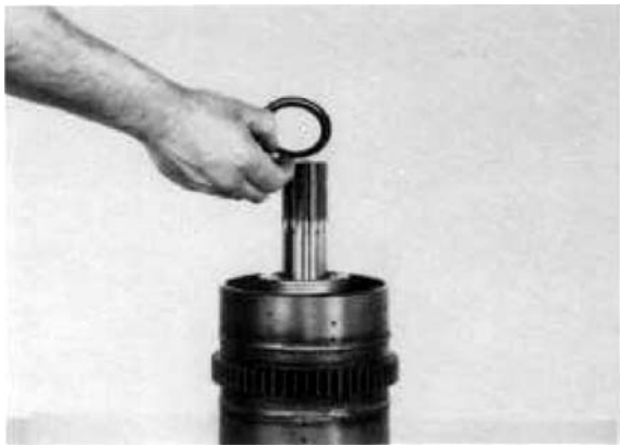
Figure 129 Remove retainer ring retaining washer.
