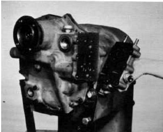
Figure 1 Remove control valve bolts and washers. Remove control valve. Use caution as not to lose detent springs and bolts.
