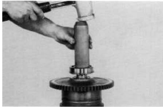
Figure 144 Install 3rd speed clutch shaft rear bearing. NOTE: Bearing outer diameter locating ring must be down.
