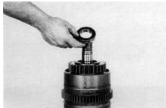
Figure 204 Install clutch gear outer bearing. NOTE: Outer bearing has a shield in it, this shield must be down.
