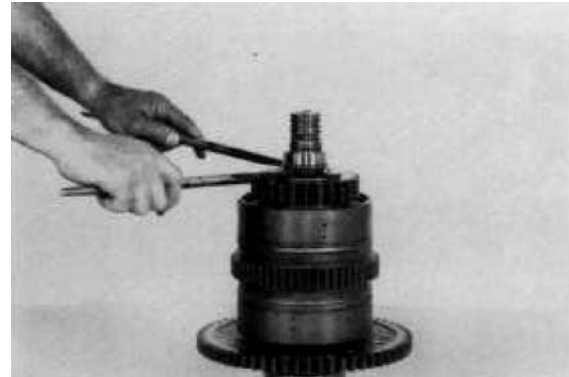
Figure 108 Pry front bearing inner race up far enough to use a bearing puller.
