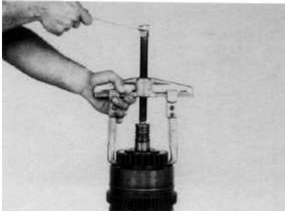
Figure 111 Remove clutch gear and outer bearing.
