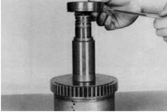
Figure 12 Install clutch shaft bearing. NOTE: Bearing snap ring groove must be down.
