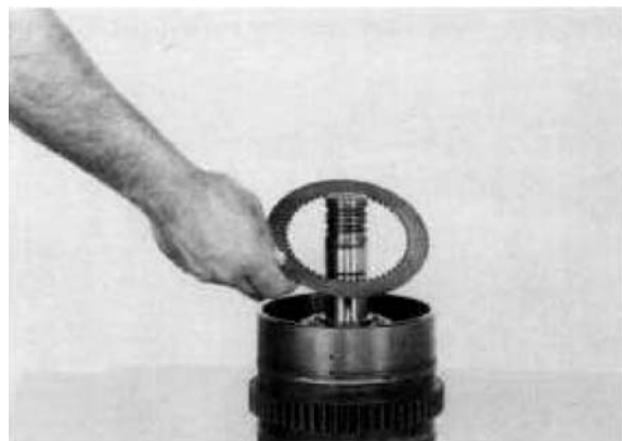
Figure 199 Install one friction disc. Alternate steel and friction discs until the proper amount of discs are installed. First disc next to the piston is steel, last disc installed is friction.
