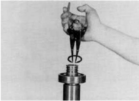
Figure 13 Install bearing retainer ring.
