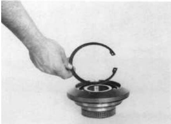
Figure 283 Install bearing retainer ring.
