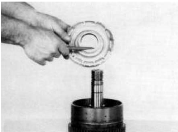
Figure 178 Remove clutch piston.
