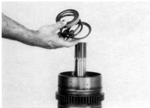
Figure 130 Remove return spring retainers and spring.
