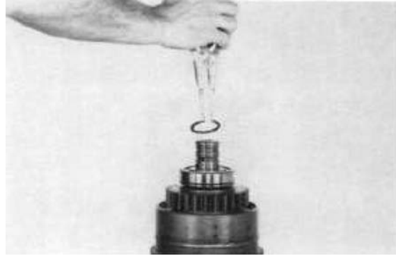
Figure 161 Install bearing retainer ring.
