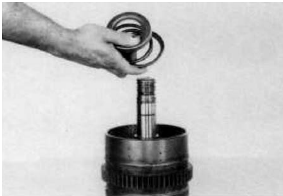
Figure 177 Remove piston return spring and retainers. See note in Figure 118.
