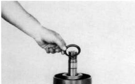
Figure 196 Position return spring retainer ring retaining washer on clutch shaft.
