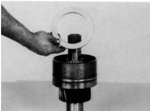
Figure 78 Remove end plate.
