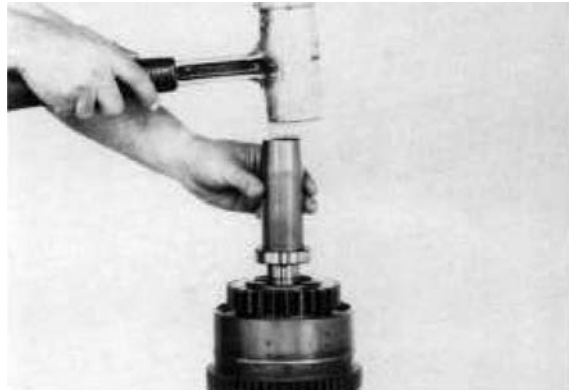
Figure 155 Install clutch gear outer bearing. NOTE: Outer bearing has a shield in it, this shield must be down.
