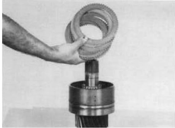
Figure 79 Remove inner and outer clutch discs.
