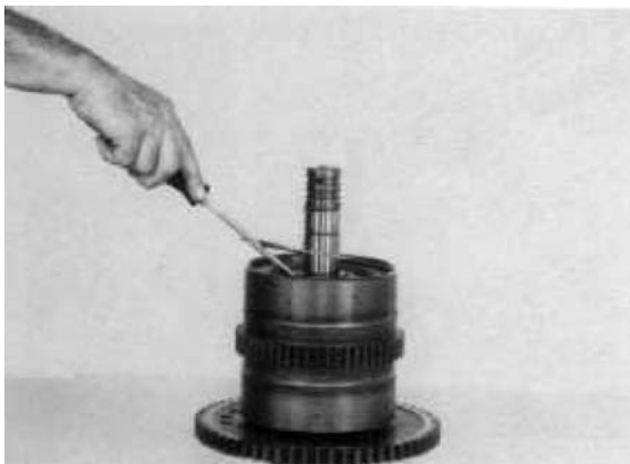
Figure 112 Remove clutch disc end plate retainer ring.
