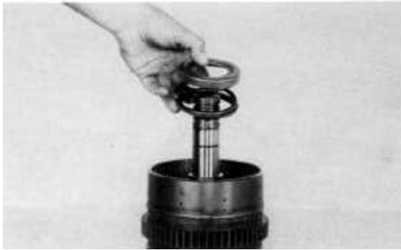
Figure 195 Position the inner return spring retainer, the return spring and outer spring retainer. NOTE: If forward and reverse clutches are modulated, assemble piston return disc springs as shown in Figure A on page 59
