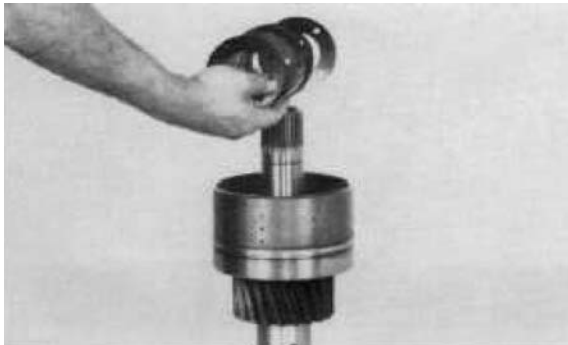
Figure 83 Remove piston return disc spring. NOTE: Disc springs in the low clutch are different than springs in the forward and reverse clutch. Do not mix low clutch springs with forward and reverse springs (see note at top of page). Non modulated units will have return springs in forward & reverse clutches.
