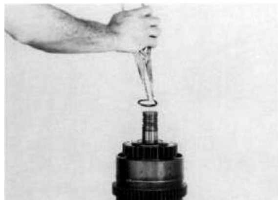
Figure 156 Install clutch gear outer bearing retainer ring.
