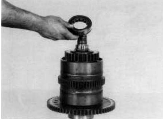
Figure 158 Position front bearing over bearing race.
