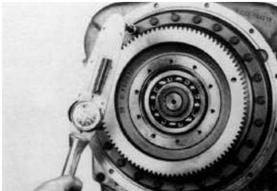
Figure 307 Install impeller cover to impeller bolts and washers. Tighten to specified torque (see torque chart).
