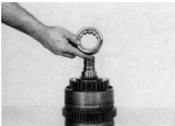
Figure 166 Remove front bearing.
