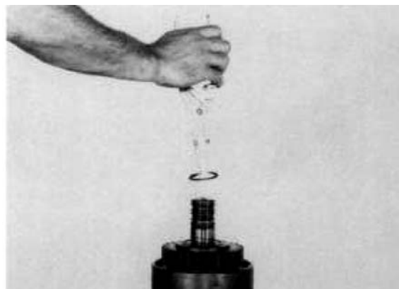
Figure 169 Remove clutch gear outer bearing retainer ring.
