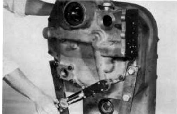
Figure 14 Support front cover with a chain fall. Install alignment studs in transmission case. Position front cover assembly on aligning studs. Turn output flange to align clutch disc hub in clutch. Do not force this operation. With front cover in position against the transmission case install cover to case bolts. Tighten to specified torque.
