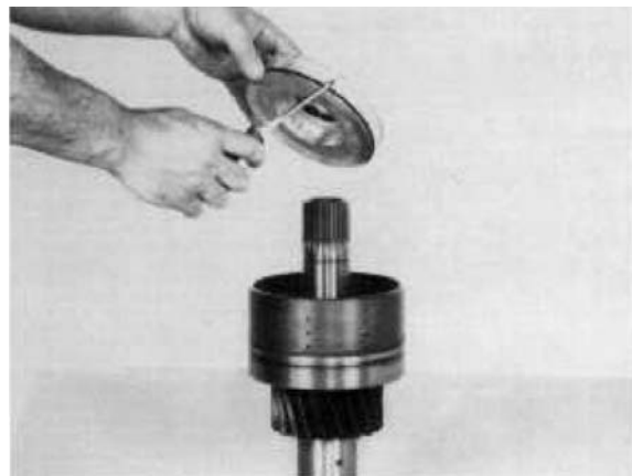
Figure 85 Install clutch piston outer seal ring.
