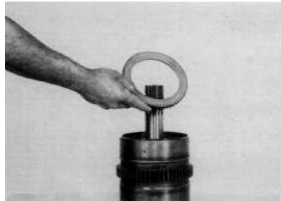
Figure 126 Remove end plate.
