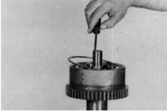
Figure 18 Install end plate retainer ring. See transmission reassembly on page 38.
