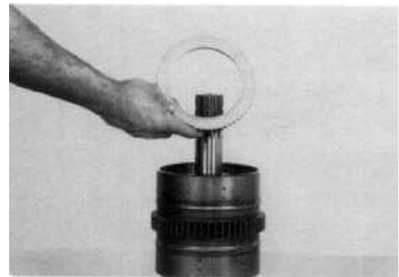
Figure 138 Install clutch disc end plate.
