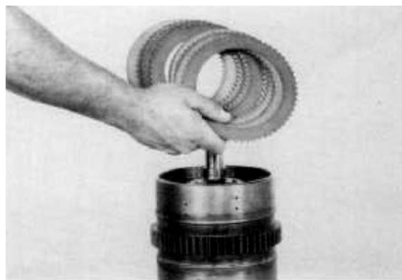
Figure 181 Remove inner and outer clutch discs.
