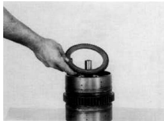
Figure 192 Install clutch disc end plate.
