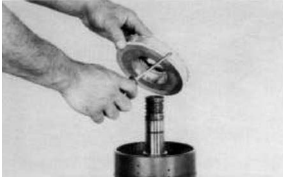
Figure 194 Install clutch piston inner and outer seal rings. Install piston in clutch drum, use caution as not to damage seal rings.
