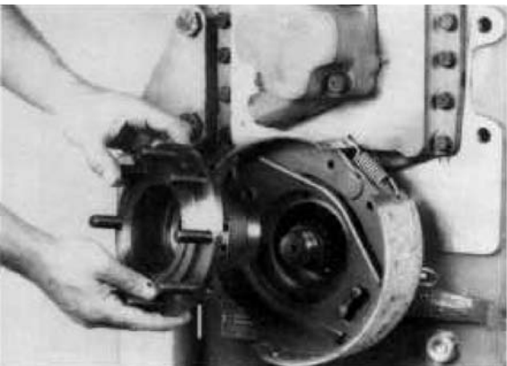
Figure 37 Remove output flange.
