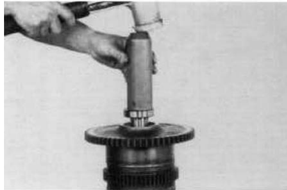
Figure 143 Install clutch gear outer bearing. NOTE: Outer bearing has a shield in it, this shield must be up.
