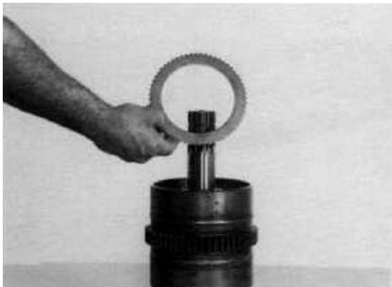
Figure 136 Install one steel disc.
