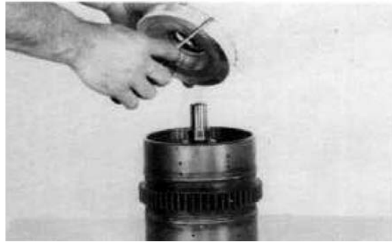
Figure 186 Install clutch piston inner and outer seal rings. Install clutch piston in clutch drum, use caution as not to damage seal rings.
