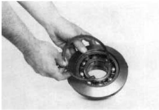
Figure 280 Remove hub bearing retainer ring.
