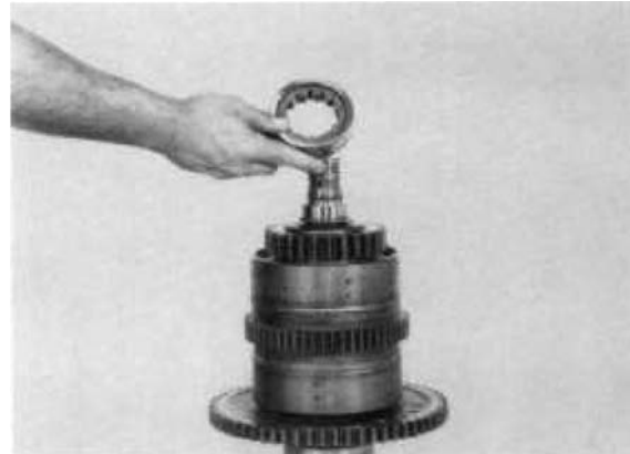
Figure 107 Remove front bearing.
