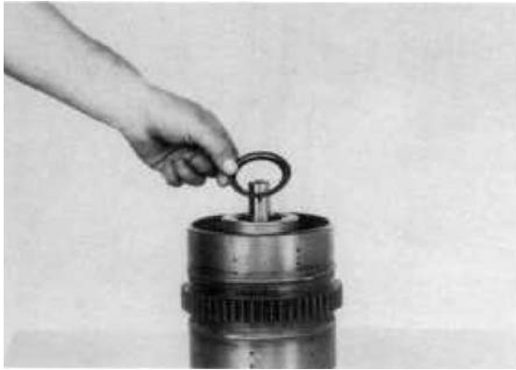
Figure 188 Position return spring retainer ring retaining washer on clutch shaft.
