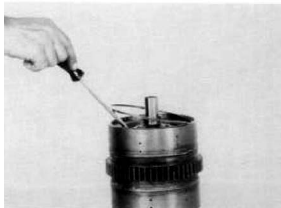
Figure 193 Install end plate retainer ring.
