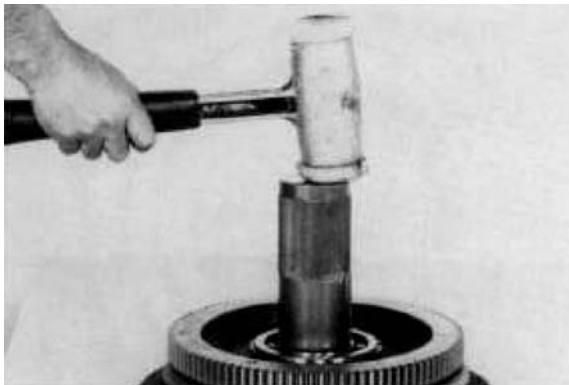
Figure 296 Install impeller cover bearing.
