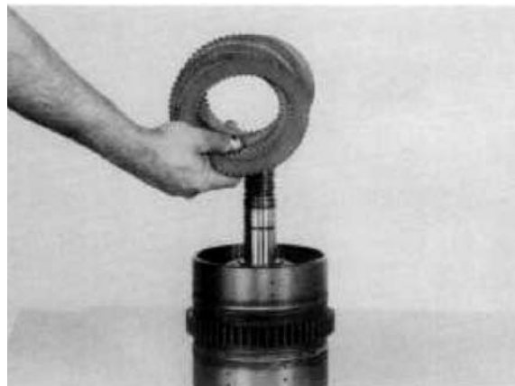
Figure 174 Remove inner and outer clutch discs.
