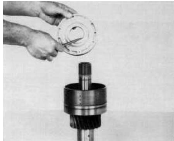
Figure 86 Install clutch piston inner seal ring. Install piston into clutch drum. Use caution as not to damage seal rings.
