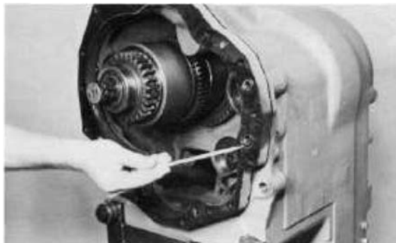
Figure 13 Install housing spacer, gasket and "O" ring seals. NOTE: Housing spacer is used with 12 plate clutch modulation only.
