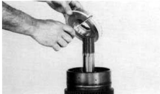
Figure 132 Install clutch piston inner and outer seal rings. Install clutch piston in clutch drum, use caution as not to damage seal rings.
