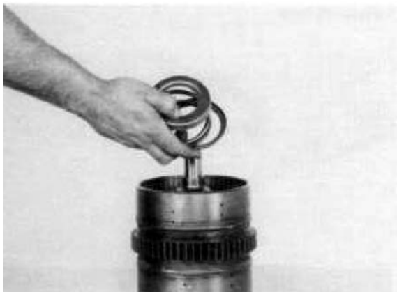
Figure 184 Remove return spring retainers and spring.
