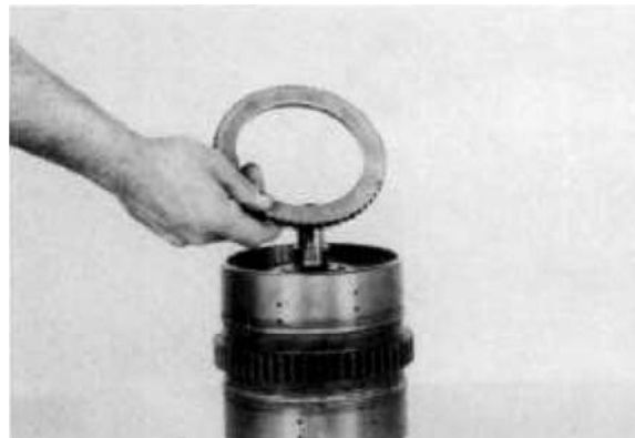
Figure 180 Remove end plate.
