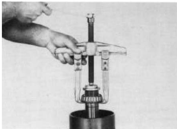
Figure 80 Remove inner taper bearing.
