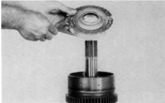
Figure 131 Remove clutch piston.
