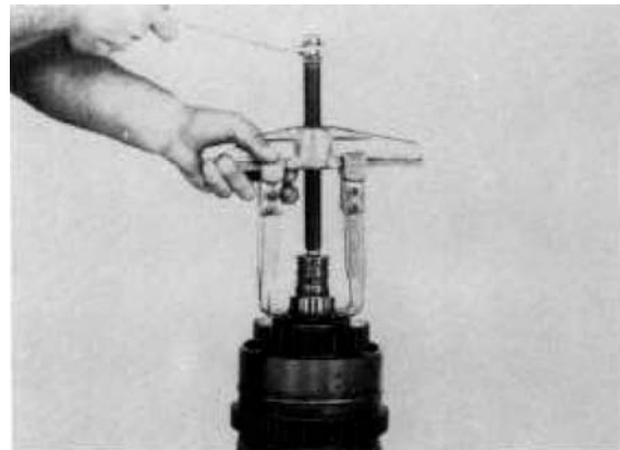
Figure 109 Remove bearing inner race.
