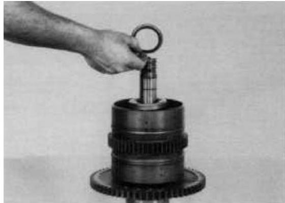
Figure 117 Remove retainer ring retaining washer.
