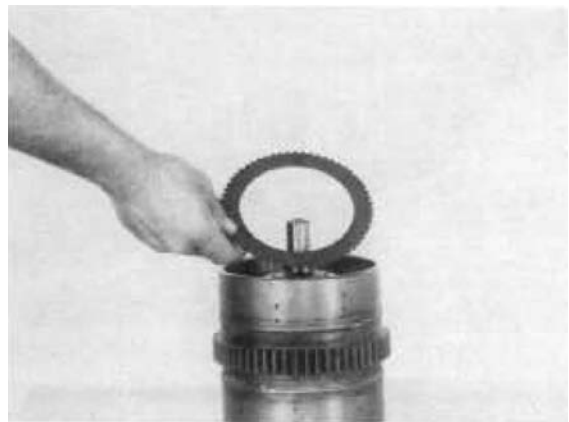
Figure 190 Install one steel disc.
