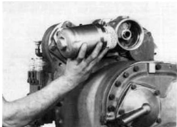
Figure 321 Install new filter element and filter housing.
