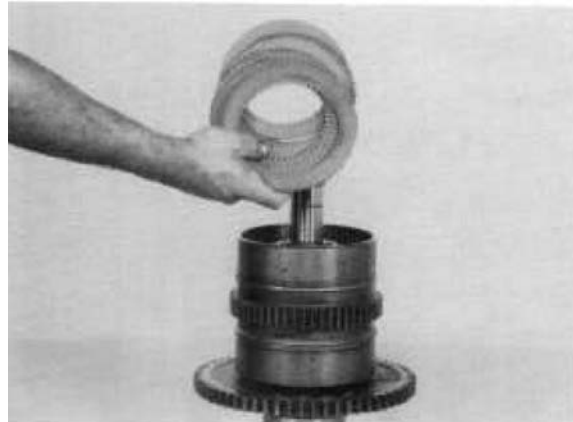
Figure 114 Remove inner and outer clutch discs.
