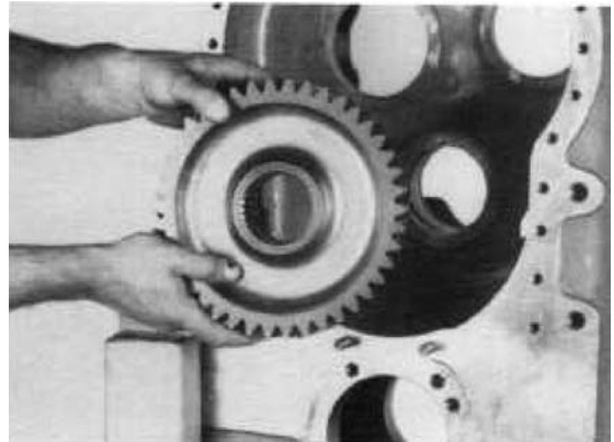
Figure 69 Remove output gear.
