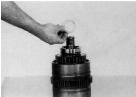
Figure 165 Remove end plate.
