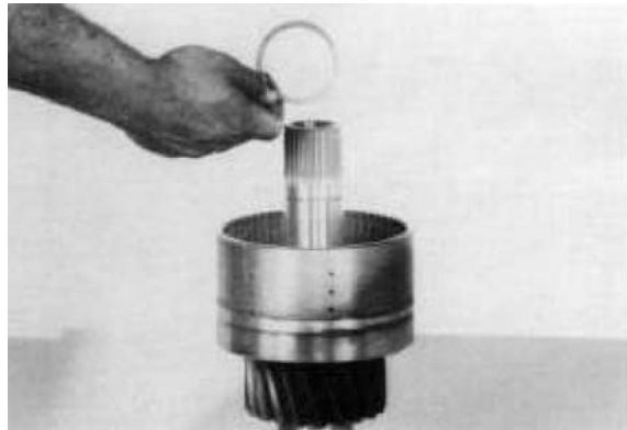
Figure 81 Remove piston return disc spring retainer ring retainer washer.
