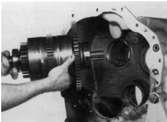
Figure 60 Remove reverse and 3rd clutch assembly.
