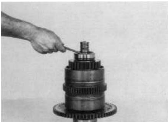
Figure 106 Remove end plate lock ball.
