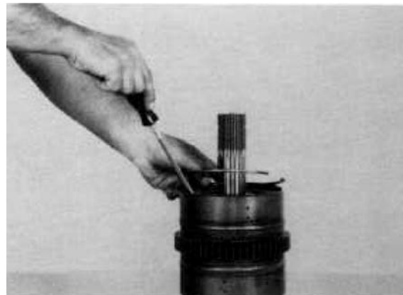
Figure 139 Install end plate retainer ring.
