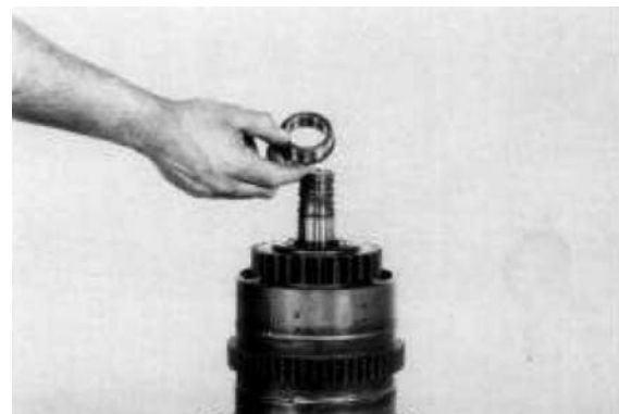
Figure 157 Install clutch shaft front bearing inner race with large diameter of race down.
