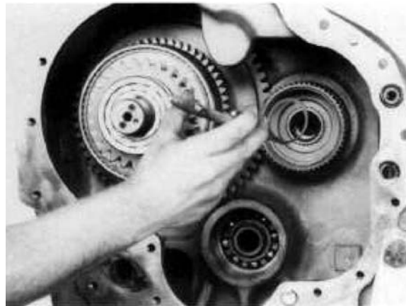
Figure 262 Install disc hub retainer ring.
