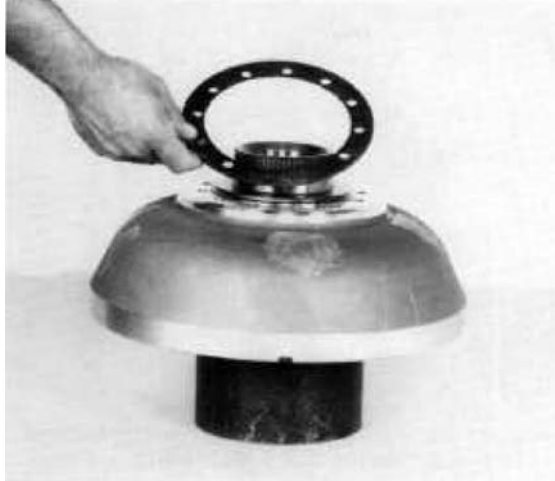
Figure 286 Position backing ring on impeller.
