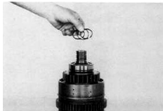
Figure 163 Remove clutch shaft piston rings. (See note in Figure 103.)
