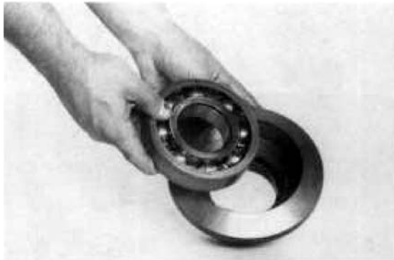
Figure 281 Remove hub bearing.
