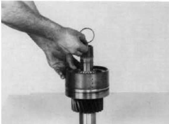
Figure 76 Remove taper bearing spacer.
