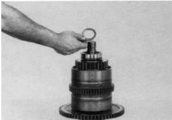
Figure 105 Remove front bearing end plate.
