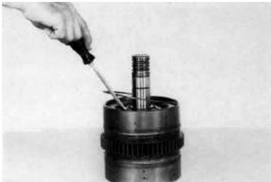
Figure 201 Install end plate retainer ring.
