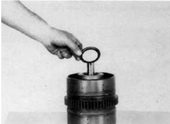
Figure 183 Remove retainer ring retaining washer.
